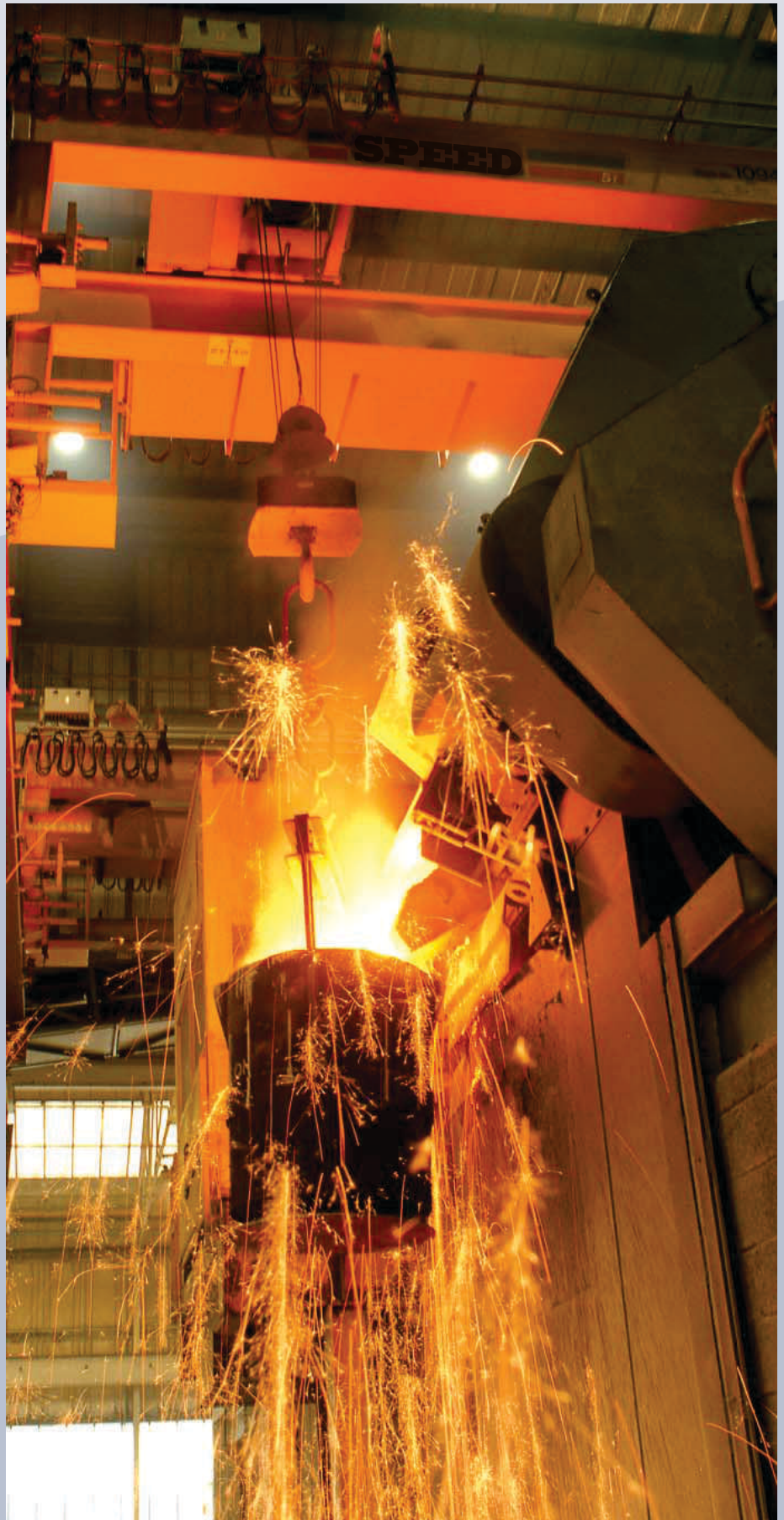
Hot metal ladle crane
