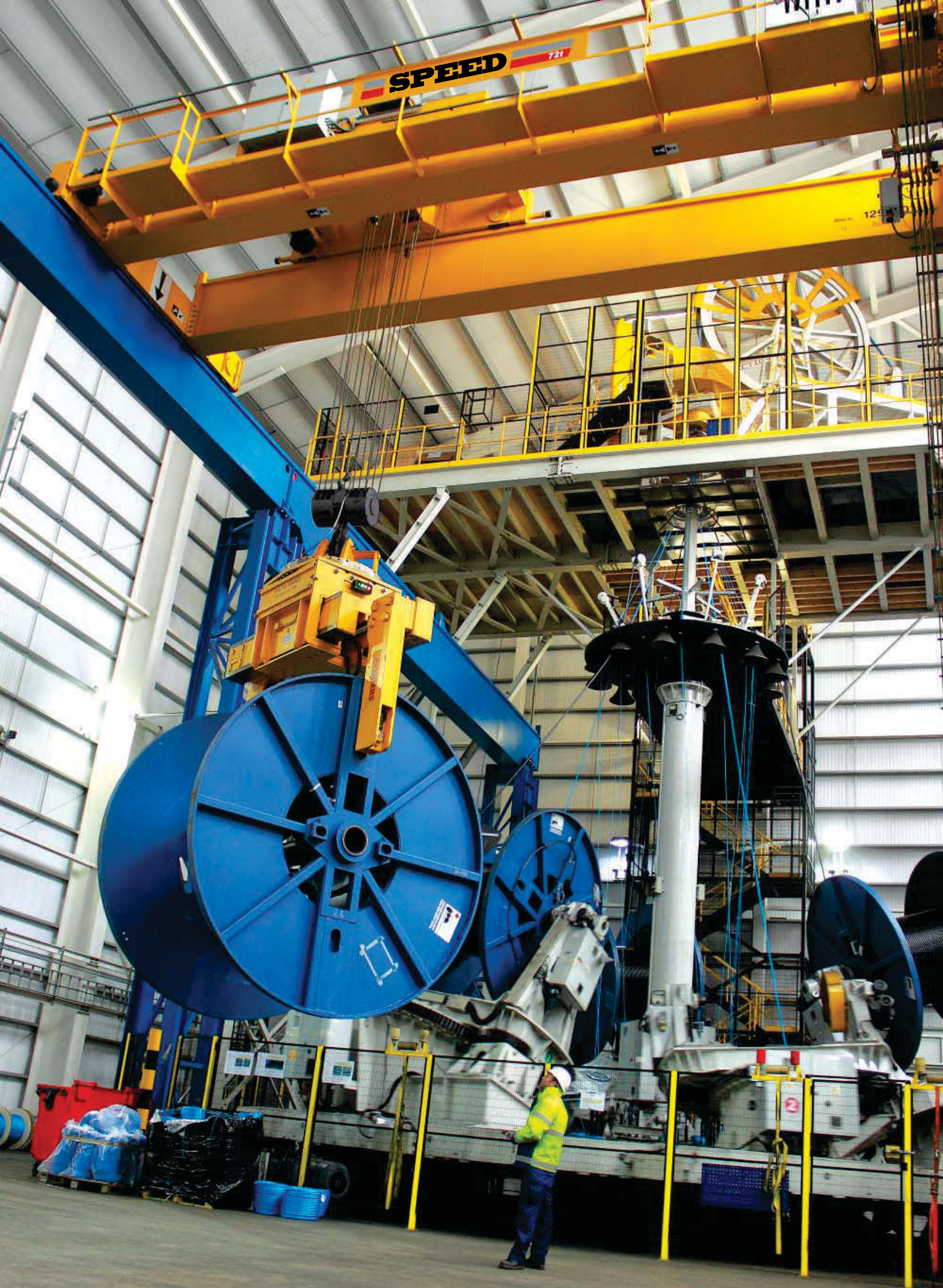
72t crane with grab
