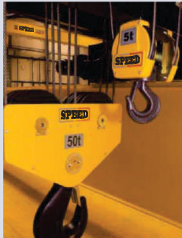
Main and auxiliary hoist
